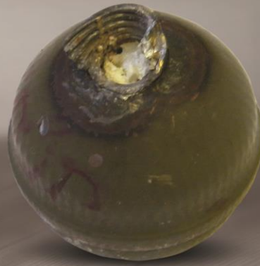
Grenade after 0.5" M20 (APIT) bullet impact
