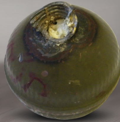
Grenade after 0.5" M20 (APIT) bullet impact
