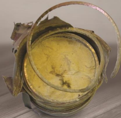
Grenade after 0.5" M20 (APIT) bullet impact
