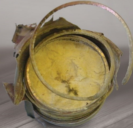
Grenade after 0.5" M20 (APIT) bullet impact
